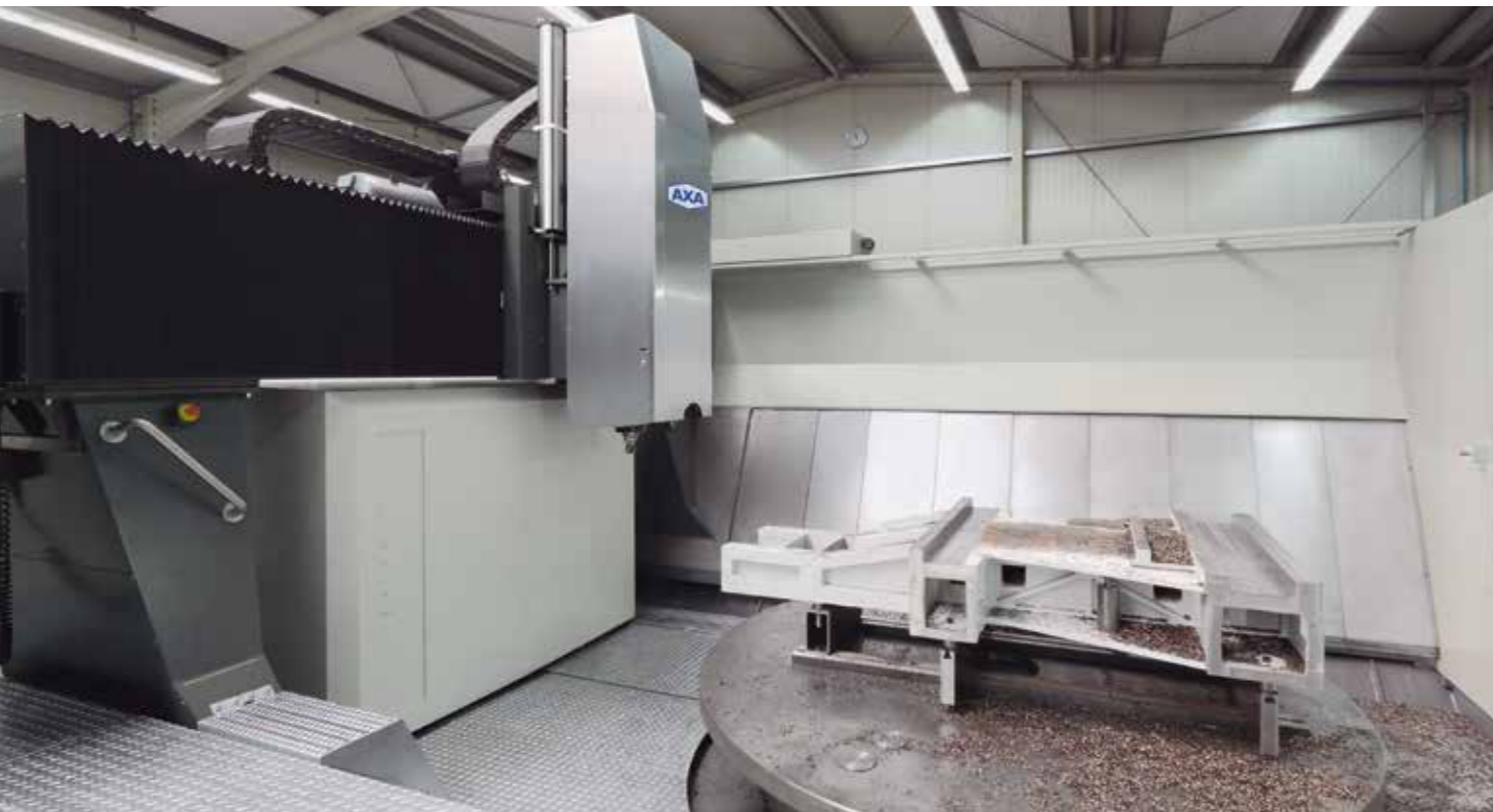
The VPC 2800 U workspace with 1-axis tilting head and rotary table is optimally accessible and visible due to its low construction
