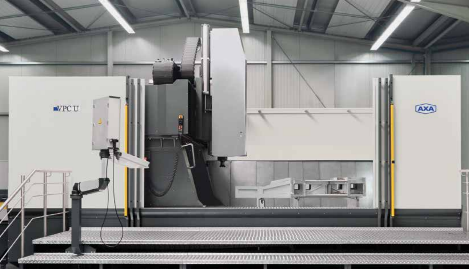
VPC 2800 U: a portal support on columns travels in the X-direction in gantry mode
