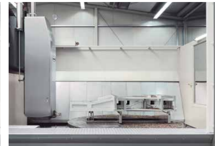
Vertical and horizontal machining of very high workpieces by the large Z travel of 1300 mm
