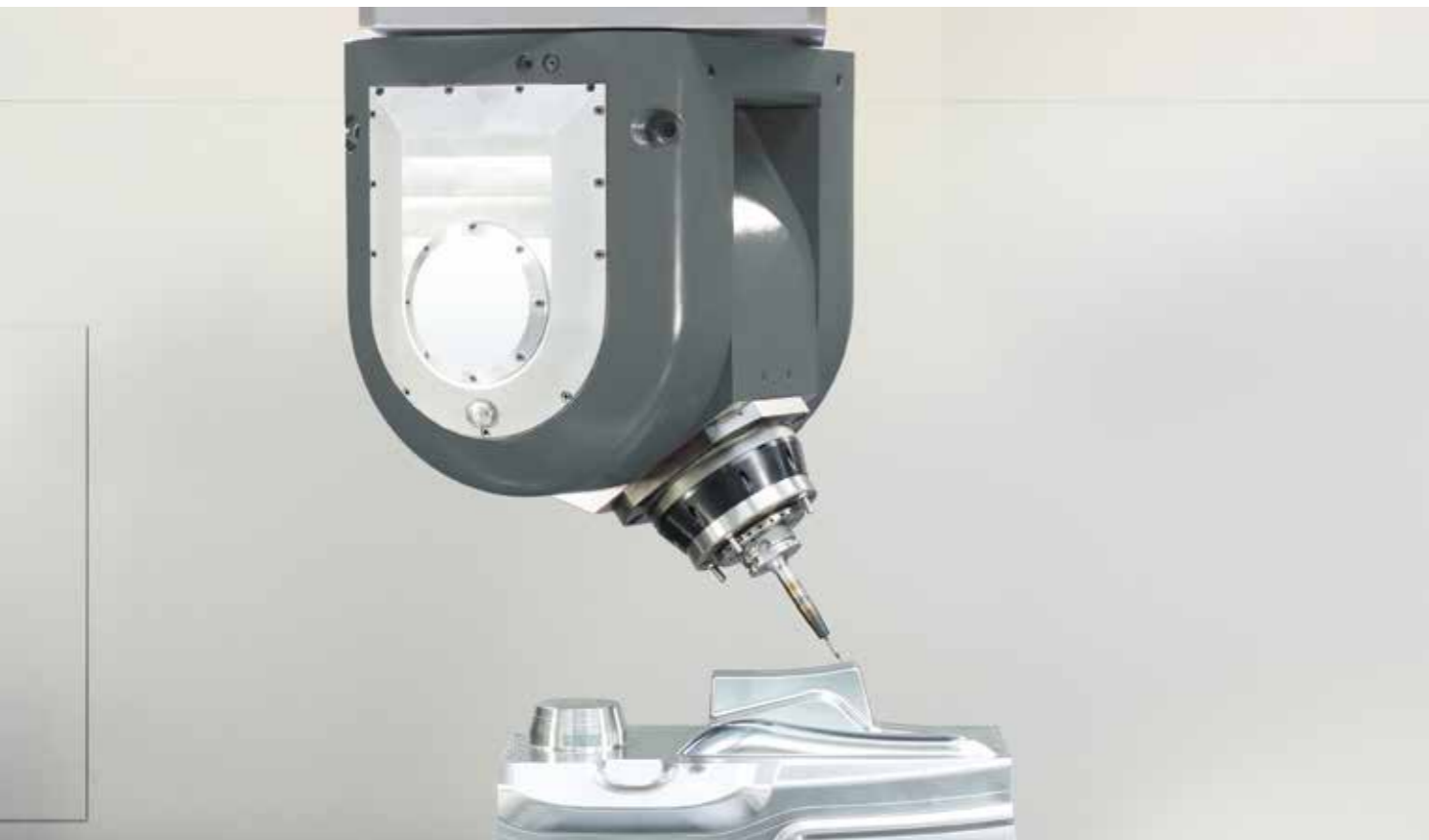
Swivelling around Z (C-axis) and X (A-axis)
