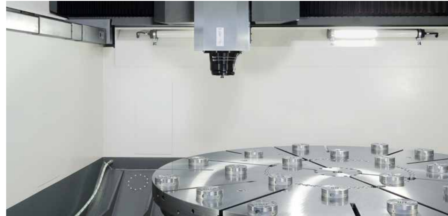
Flexible zero point clamping systems, adapted according to requirement, guarantee the precise workpiece alignment and clamping
