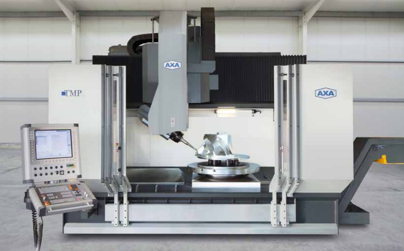
Impeller processing on AXA 5-axis gantry machining centre TMP
