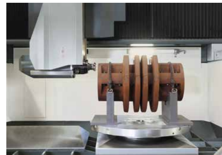
High precision manufacturing by work-and-turn processed workpieces
