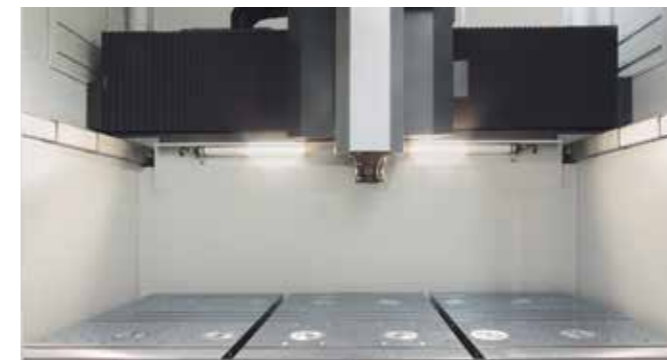
Zero point clamping system set in table for exact and quick loading of clamping equipment and tool pallets
