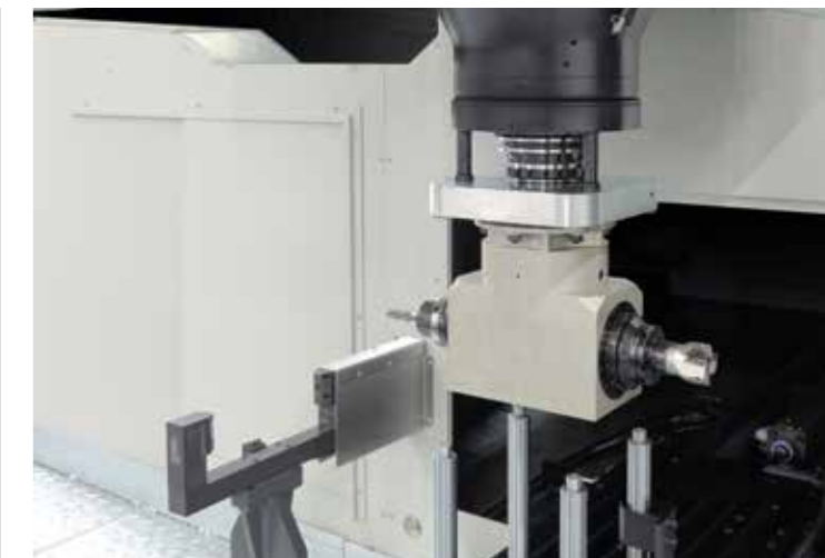
Vertical and horizontal machining of very high workpieces by the large Z travel of 1300 mm
