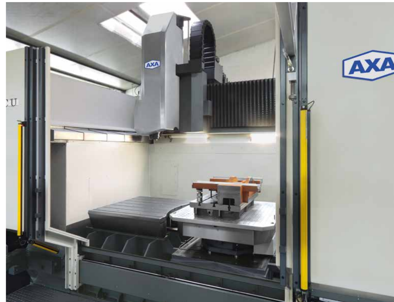
Workpiece machining on clamped pallet with the VPC
