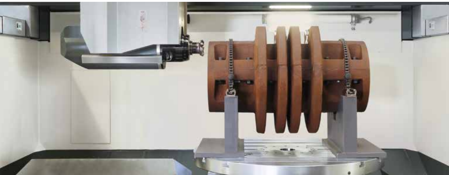
Milling processing of a coupling on the TMP
