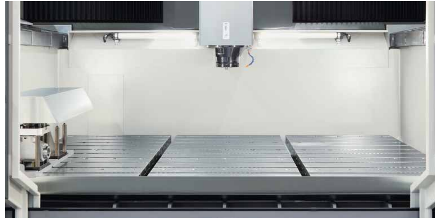
Additional pick-up station at the edge of the working area for use of angular heads and oversized tools
