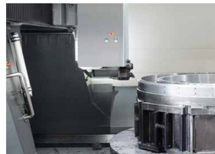
Turning – the separate clamping unit for turning tools ensures high stability and avoids stress on the main spindle bearing
