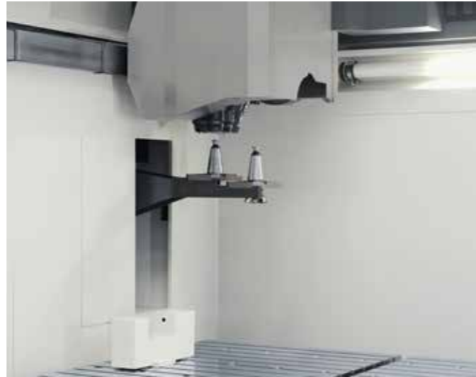
The double gripping arm for short tool changing times
