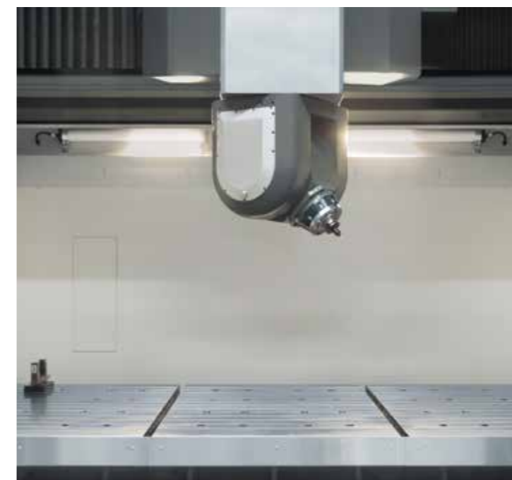
2-axis tilting head of the VPC 45 DASK: the entire head tilts around the Z-axis (C-axis) with a tilting range of \pm 360^\circ while the spindle can be tilted in the fork around the X-axis (A-axis) in the tilting range of \pm 110^\circ
