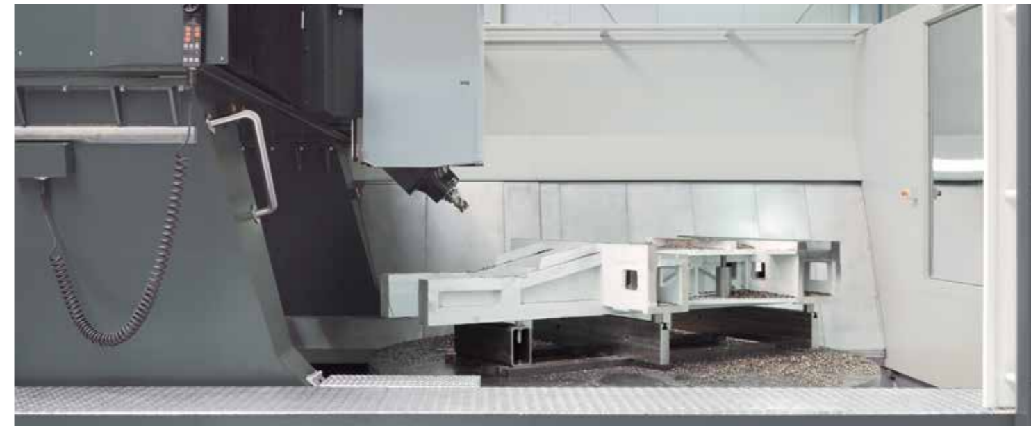
5-sides and 5-axis machining of large cubic workpieces by VPC 2800 U tilting head and rotary table
