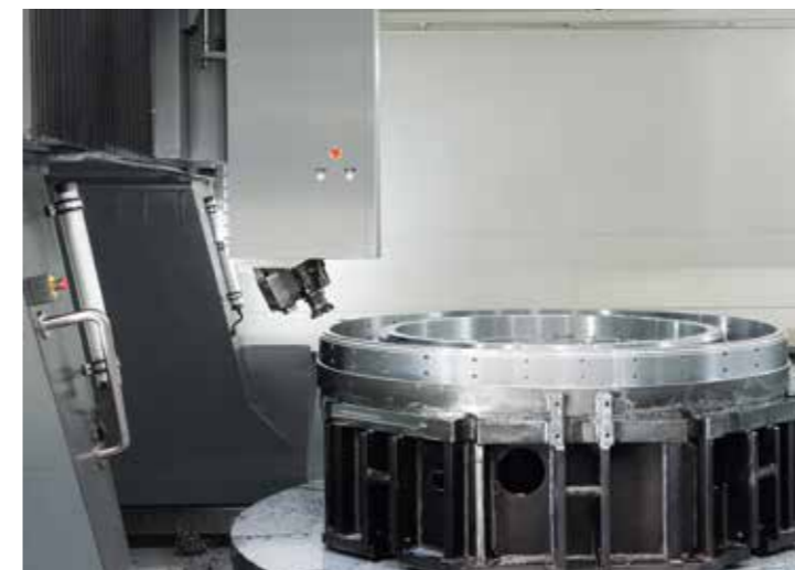
VPC 2800 U with optional full enclosure – when the bellows roof is open, the working area is accessible for loading from above
