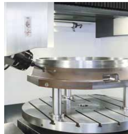
Processing of a rotary table housing in a tilted plane
