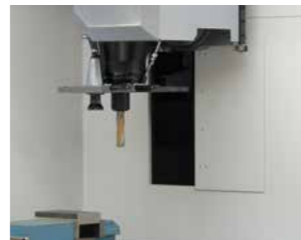
Short tool changing times by double gripping system
