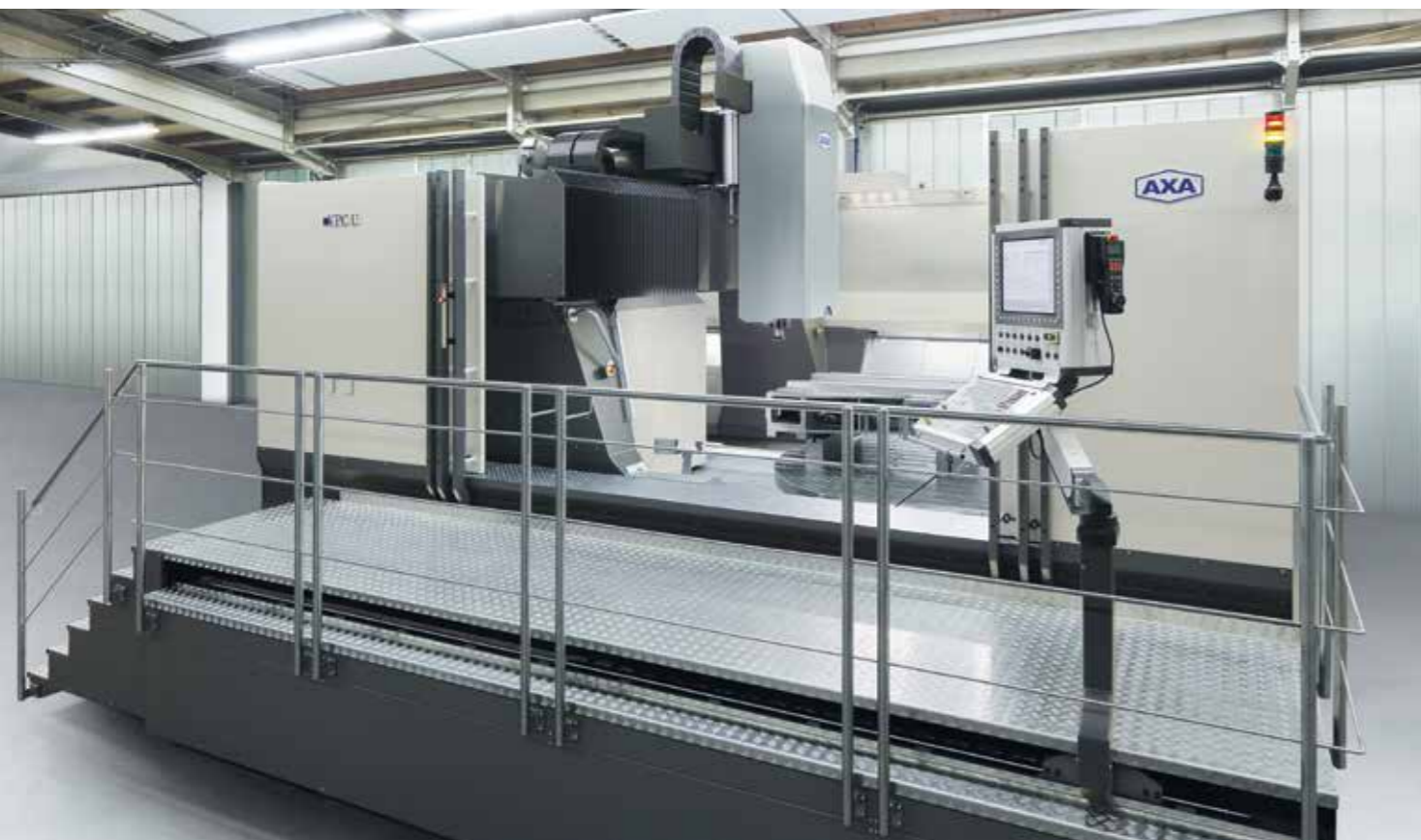
Excellent machine accessibility with crane loading possibility by the optional complete covering with automatic doors and automatically opening bellows in the roof section
