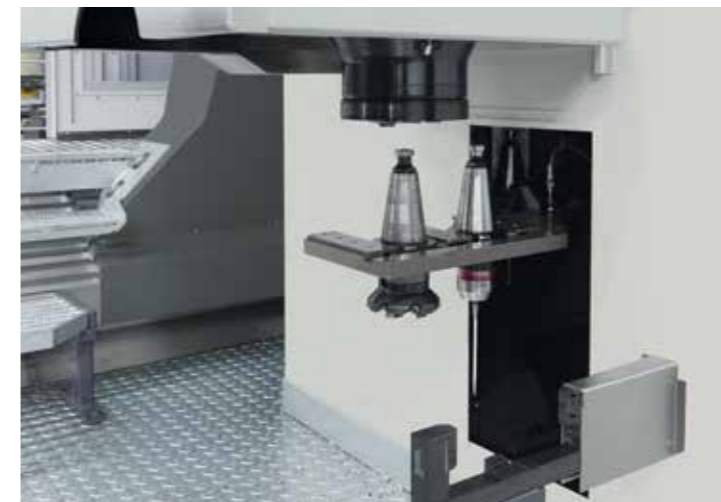
Tool changer systems are set in a protected housing at the rear under the portal
