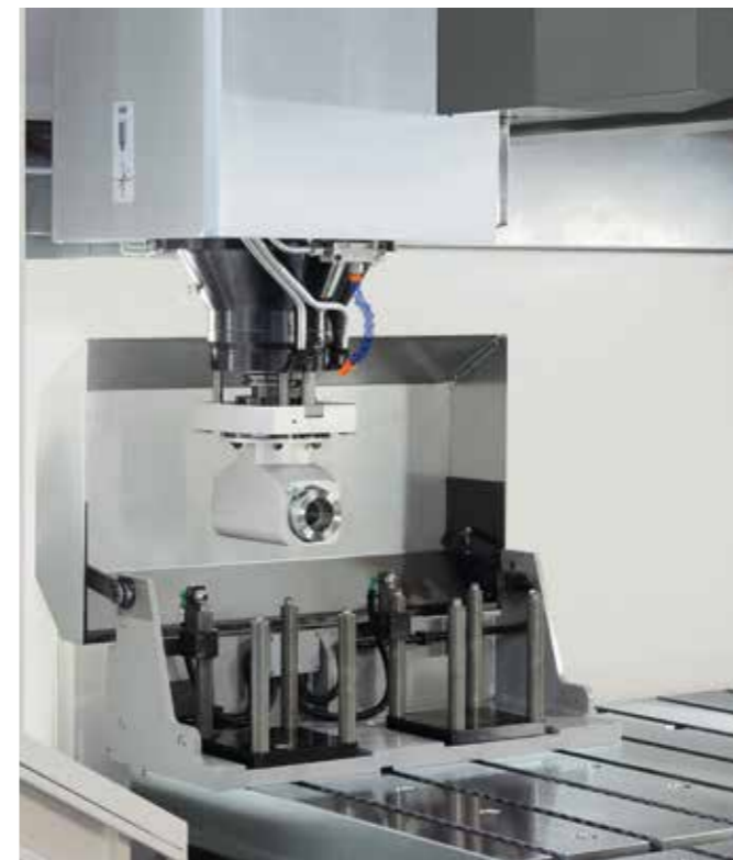
Pick up of one or more angular heads by individually adapted pick-up station
