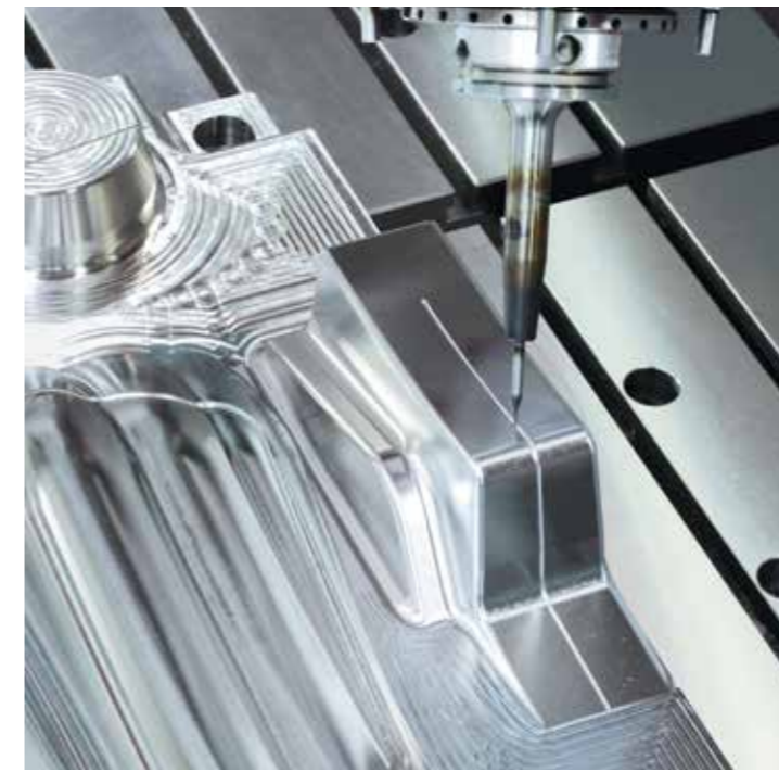
Finishing and multipass milling of surfaces – highest form and contour accuracy due to high speed ranges
