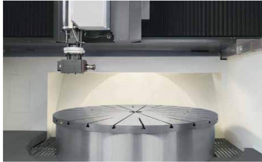
For smaller ring diameters – additional angular heads for inside machining can be added
