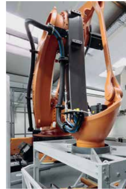
Pick up of workpiece pallet by a special gripping system
