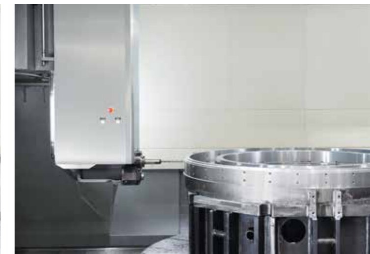
VPC 2800 U with optional full enclosure – when the bellows roof is open, the working area is accessible for loading from above
