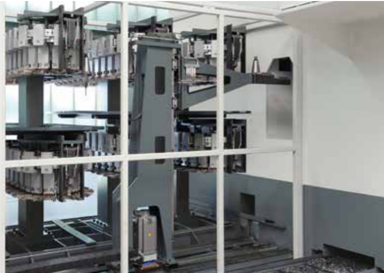
The tool changing system is well protected, side-mounted at the back of the working area
