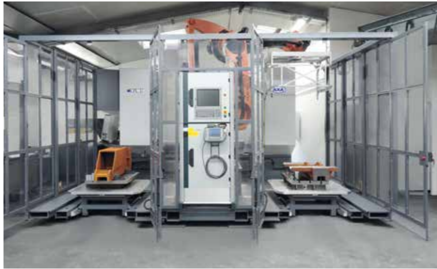
VPC with two pallet positions ahead for machine loading
