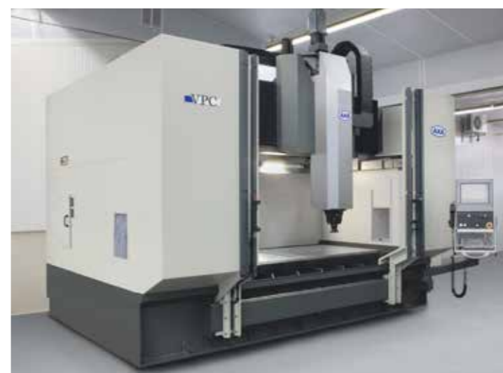
The machine has a complete encasement as standard that opens from above
