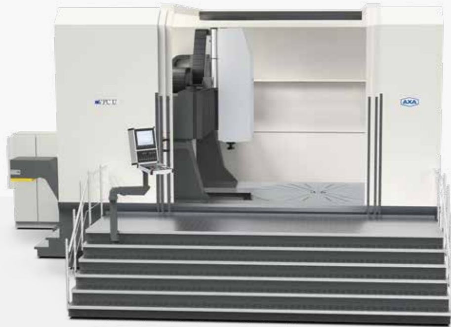
The AXA gantry machining centres VPC 2800 U, VPC U and VPC in compact form, when compared with travelling column machines, achieve much higher cross travels (Y-axis) without any limitations on exactness and stiffness
