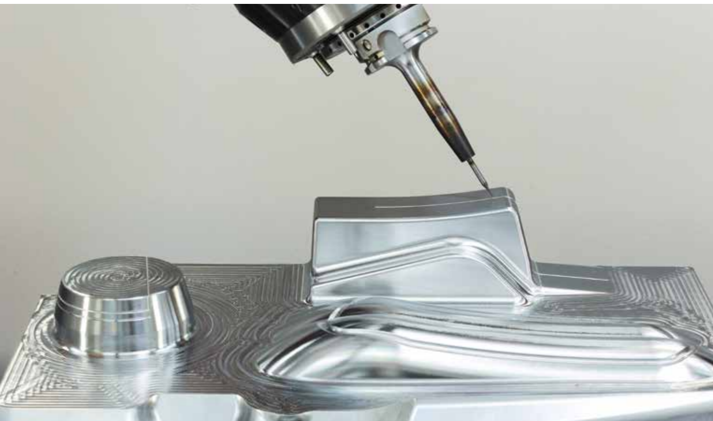
The torque drive provides the fork head with utmost acceleration
