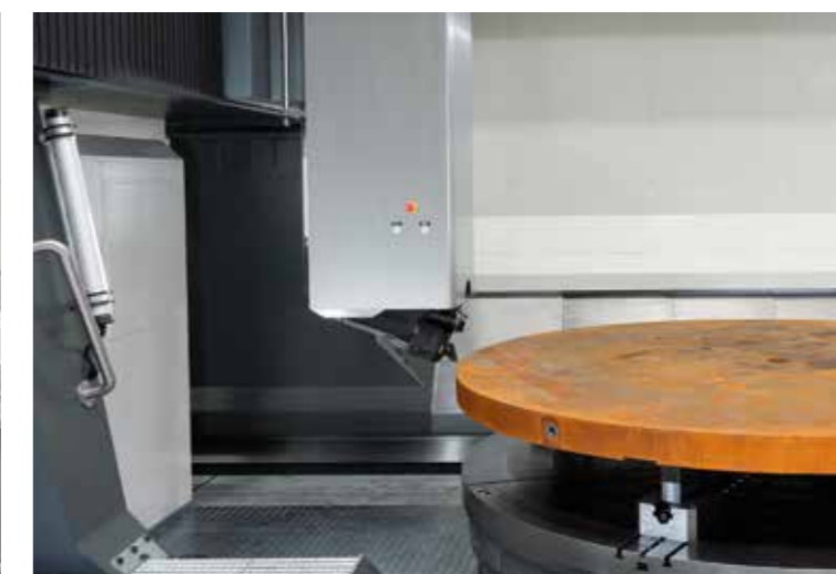
Turning – the separate clamping unit for turning tools ensures high stability and avoids stress on the main spindle bearing
