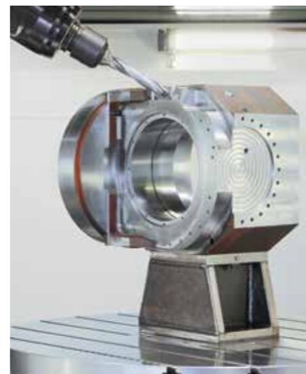
Supreme precision: 5 sides drilling and milling processing of an AXA tilting spindle head body that is ideal for processing parts in one setting
