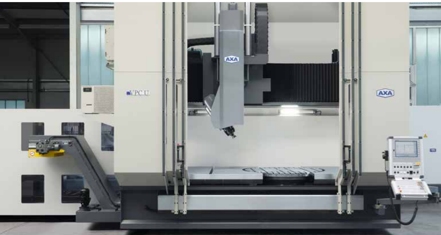
Side-mounted tool magazine towers for various tool clamping systems that can be extended as required
