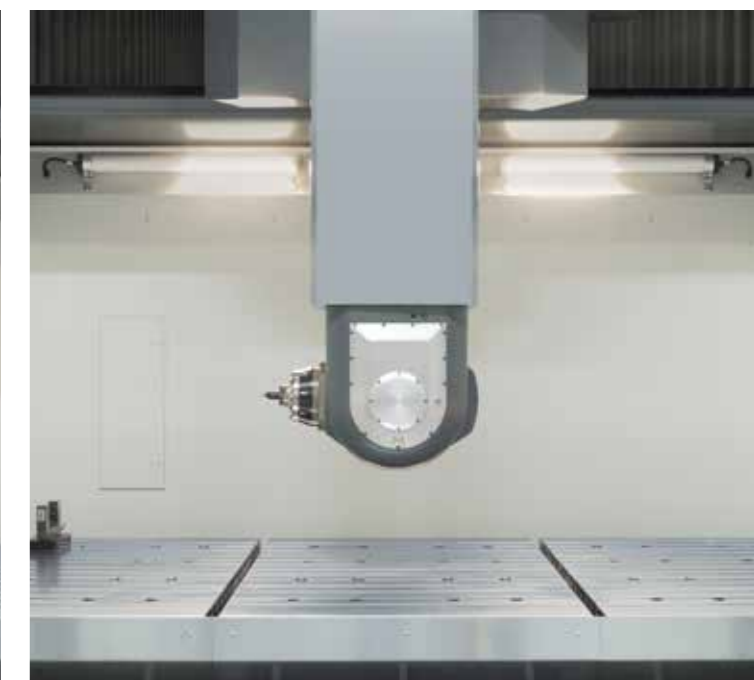
2-axis tilting head of the VPC 45 DASK: the entire head tilts around the Z-axis (C-axis) with a tilting range of \pm 360^\circ while the spindle can be tilted in the fork around the X-axis (A-axis) in the tilting range of \pm 110^\circ
