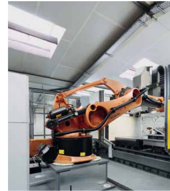
Workpiece pallet implementation in machining by centre zero point clamping system
