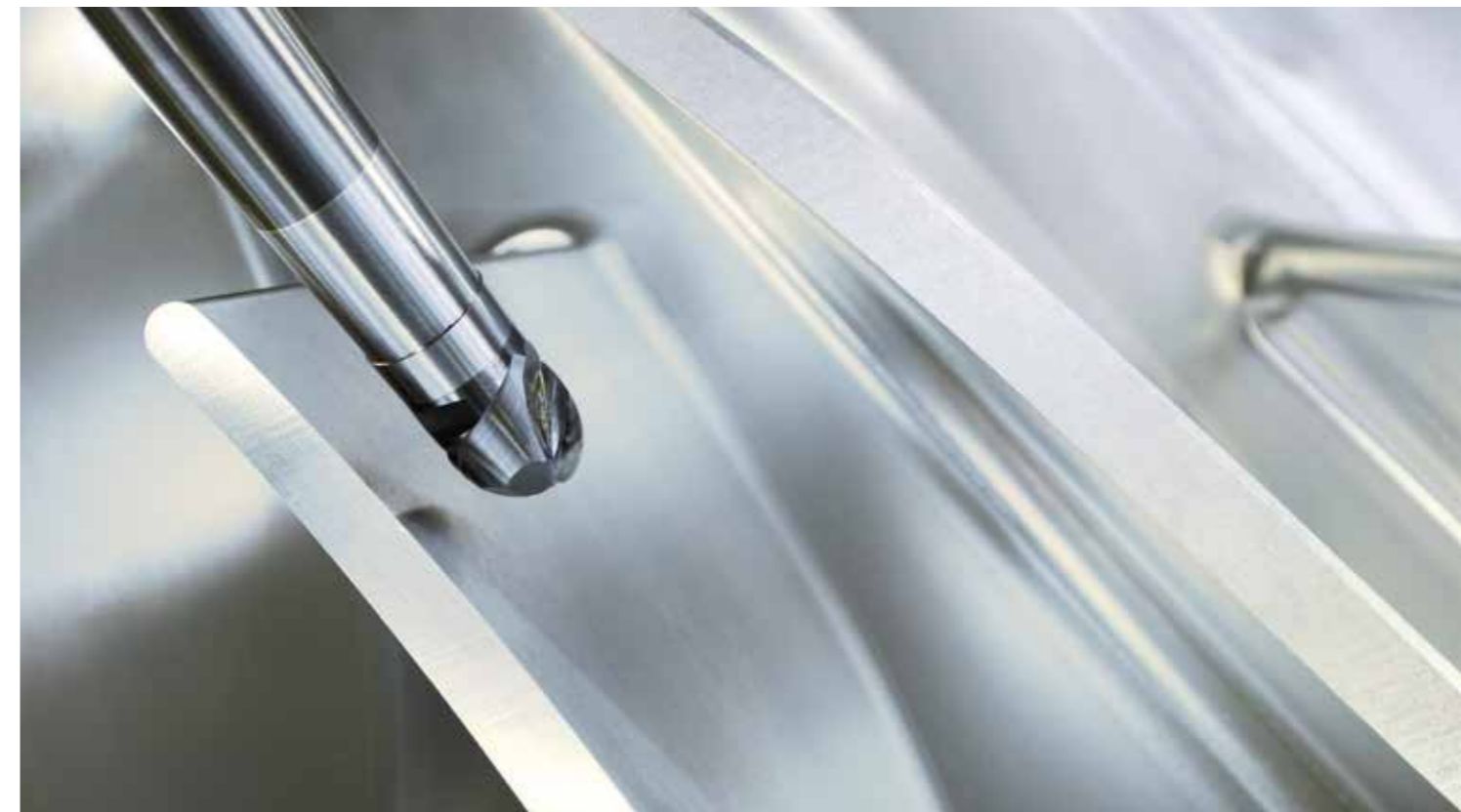
Finishing by a ball-end cutter
